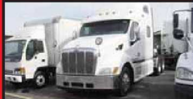
2006 and 2007 PETERBILT 387 CONDO, double bunk, Cat C15-475hp, 10spd, jake, cruise, full fairings, aluminum all around, air slide 5th wheel, STARTING AT $35,900
